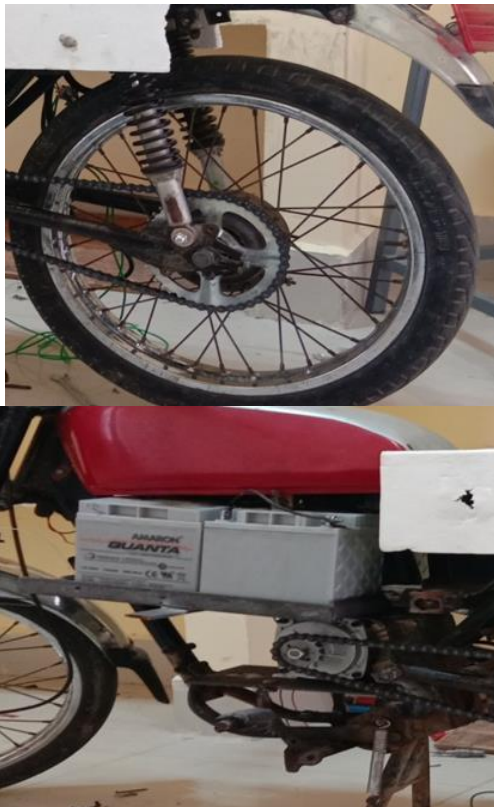
Figure 2. Rear Wheel Setup Figure 3. Battery and Motor Setup
